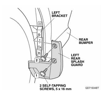
10. Secure the left rear splash guard to the rear inner under cover with one clip.
