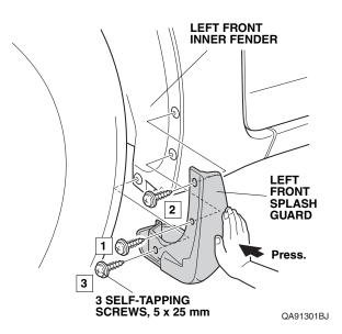
4. Turn the steering wheel fully clockwise, and repeat steps 2 and 3 to install the right front splash guard on the right side of the vehicle.
